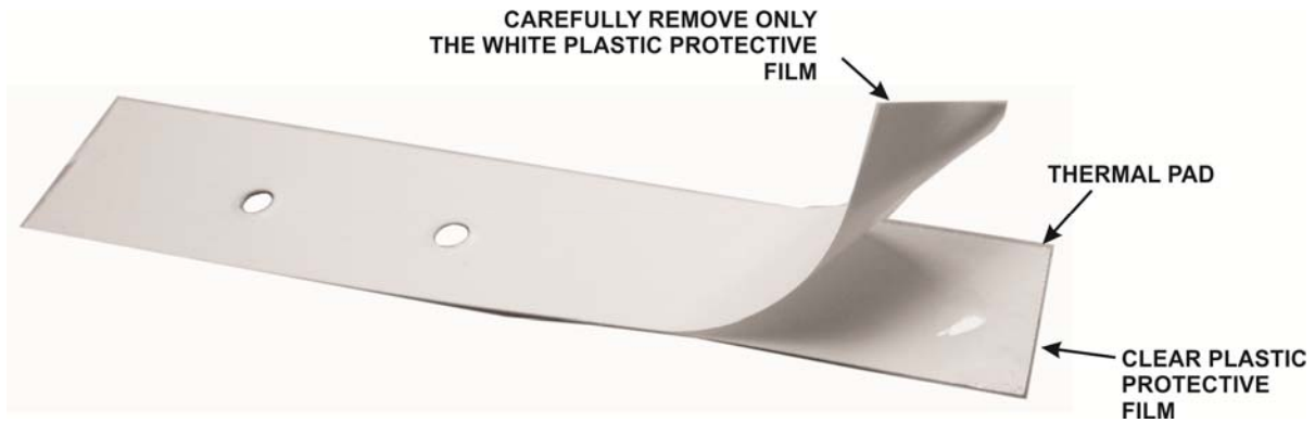
Figure 5. Preparing the Thermal Pad.
